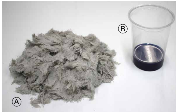
The liquid hardener component Biresin® L90 (B) is coloured blue for safe mixing control.
