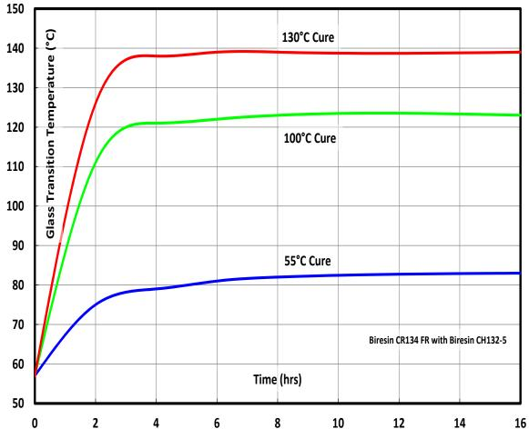
The test specimens were produced from 3 mm thick pure resin. Before the above postcuring, the samples were cured for 7 days at 23°C. When curing a composite part, the whole of the part (including the very middle of the laminate) needs to see the cure temperature.
